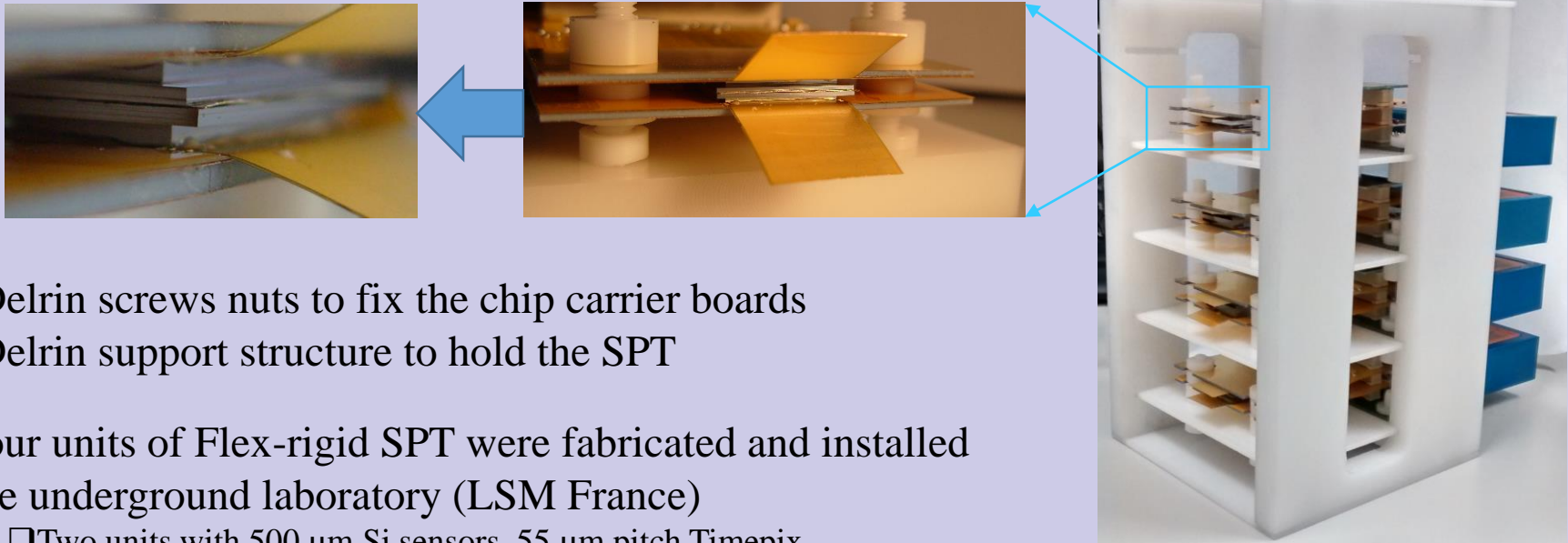
Four units of Flex-rigid SPT arranged with Delrin support structure
