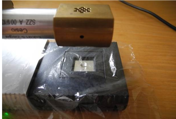
Figure 58: The setup for demonstration of the absorption of radiation in a water drop. The sensor is in the horizontal position, above it is a piece of food wrapping foil with a drop of water and above the center of the sensor is the radiation source. For a better visibility of the drop is the source in this picture placed higher than in actual measurement.
